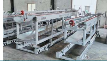
Pig Handling System
