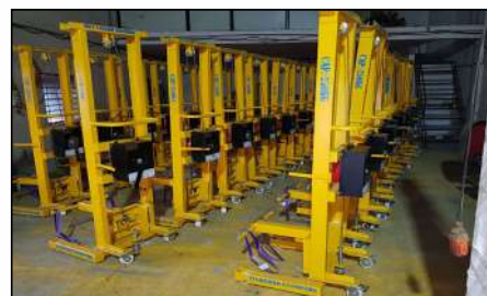
ACB Breaker trolley
